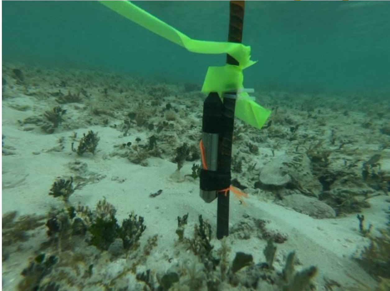
Figure 7.14. Image of tide gauge at Leeward Harbour.
